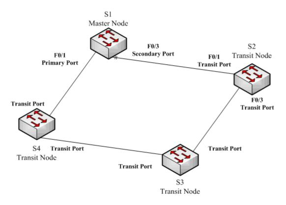
Figure 2.1 Security settings of EAPS Ethernet ring
